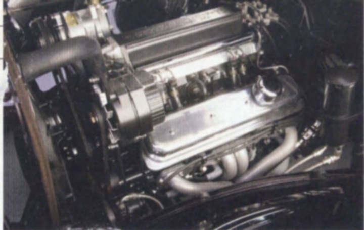
Bob's panel is powered by a GM Performance Parts Ram Jet 350, backed by a 4L60E overdrive transmission.
