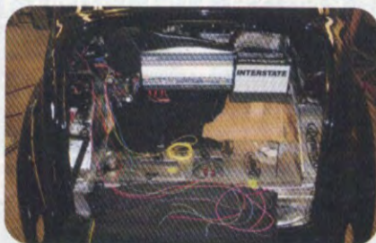
Nearing the end of the electrical system's assembly we see the trunk of the Tudor sedan will be the nerve center. The Vintage Air evaporator is mounted to the rear wall of the interior. Cool air will vent in the package tray behind the rear seat. The Air Ride air tank is mounted to the passenger side of the trunk. Note the generous use of Dynamat insulation. All of the mechanicals and wiring will be hidden by upholstered panels created by Fast Ed's Upholstery located in Torrance, California.
