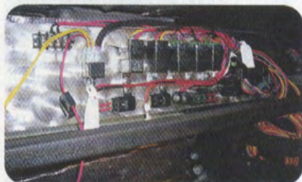
Much of this area will become covered with A/C hoses that connect to the billet aluminum firewall bulkhead (below the dash on the passenger side).
