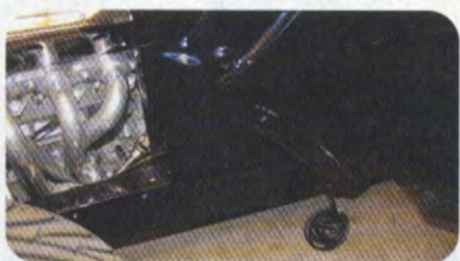
The coiled cable at the bottom of the fender well will eventually be installed to provide important emergency access (mechanical latch) to the sedan's interior in the remote event that there should be a dead battery.
