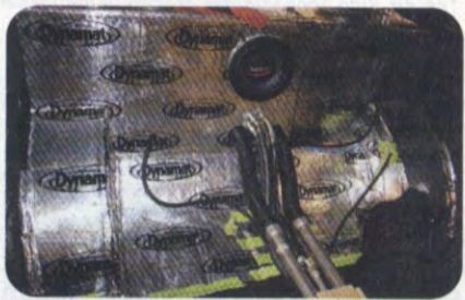
Cool air from the rear-mounted A/C evaporator will also be directed to the front of the sedan's interior through insulated pipes housed in the center console.
