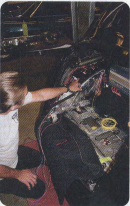
Robert points out the location of the primary fuse panel. Also visible is the trunk-mounted hydraulic arm that will open and lift the sedan's large trunk lid.
