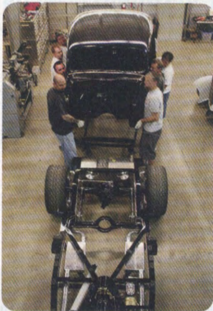
Every crew member in the Hot Rods & Hobbies shop was called on to lift the freshly painted body off the paint dolly onto the rolling chassis. The body was slightly lighter without the dash, doors and trunk lid.
