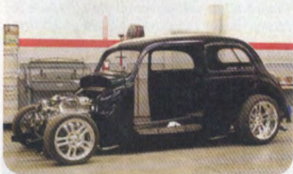
Once on the chassis the HR&H crew stepped back to check the stance and the wheel/tire fitment before the next phase of installing the electrical system began.
