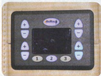
The Air Ride Technologies control panel is mounted close at hand in the center console in front of the power window switches.
