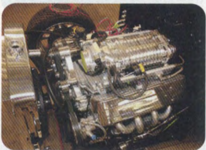
A Street & Performance LS-1 and 4L60E overdrive transmission were in the chassis, cooling will be handled by an aluminum radiator.
